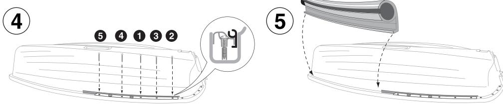
Step 4: Reinstall screws into gunwale cap. DO NOT TIGHTEN COMPLETELY
