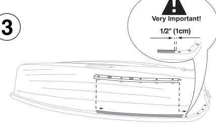
Step 3: Reinsert gunwale cap into the gunwale with the track firmly against the hull of the boat.
