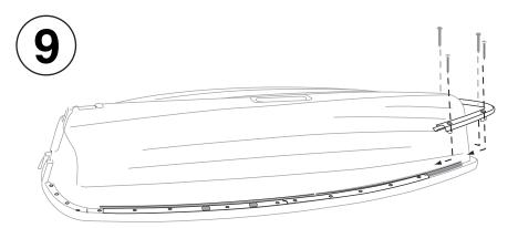
Step 9: Insert bow gunwale cap unto the gunwale, insert screws and hand tighten until snug.
