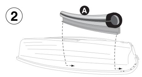
Step 2: Insert track into gunwale with the capped end facing the stern of the boat.
