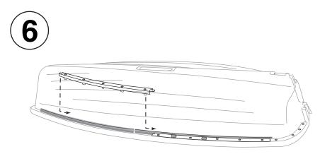
Step 6: Reinsert gunwale cap into the gunwale with the track firmly against the hull of the boat.
