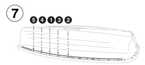
Step 7: Reinstall screws into gunwale cap, hand tighten all gunwale screws until snug.
