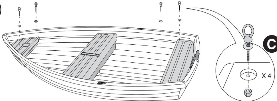
Step 10: Remove 2 seat bolts from the bow and stern seats. Replace with davit lifting eyebolts.
