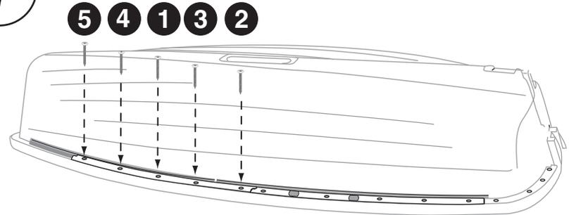
Step 7: Reinstall screws into gunwale cap, hand tighten all gunwale screws until snug.
