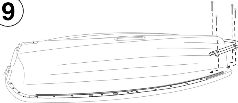
Step 9: Insert bow gunwale cap onto the gunwale, insert screws and hand tighten until snug.
