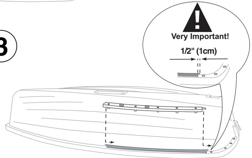
Step 3: Reinsert gunwale cap into the gunwale with the track firmly against the hull of the boat.
