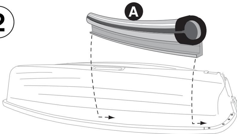
Step 2: Insert track into gunwale with the capped end facing the stern of the boat.
