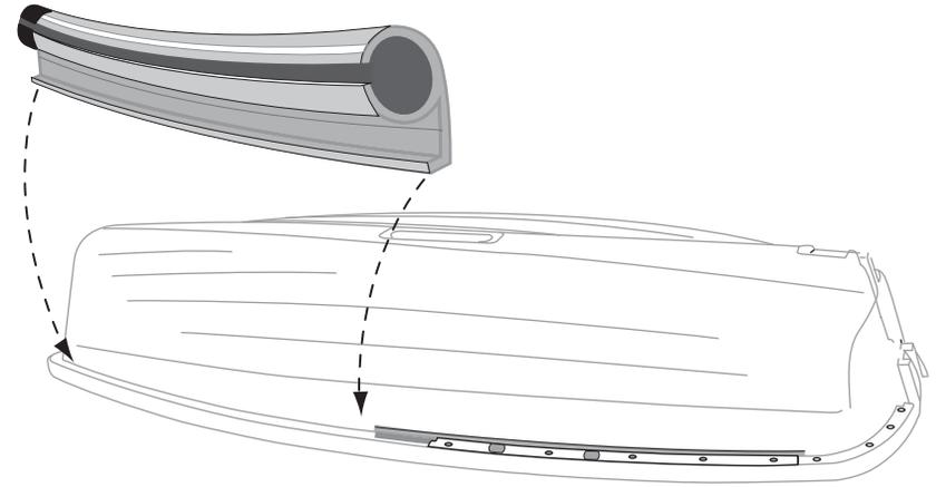
Step 5: Insert track into gunwale with the capped end facing the bow of the boat.
