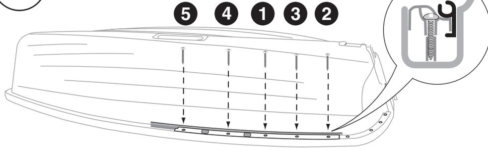
Step 4: Reinstall screws into gunwale cap.
