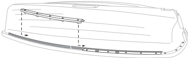
Step 6: Reinsert gunwale cap into the gunwale with the track firmly against the hull of the boat.
